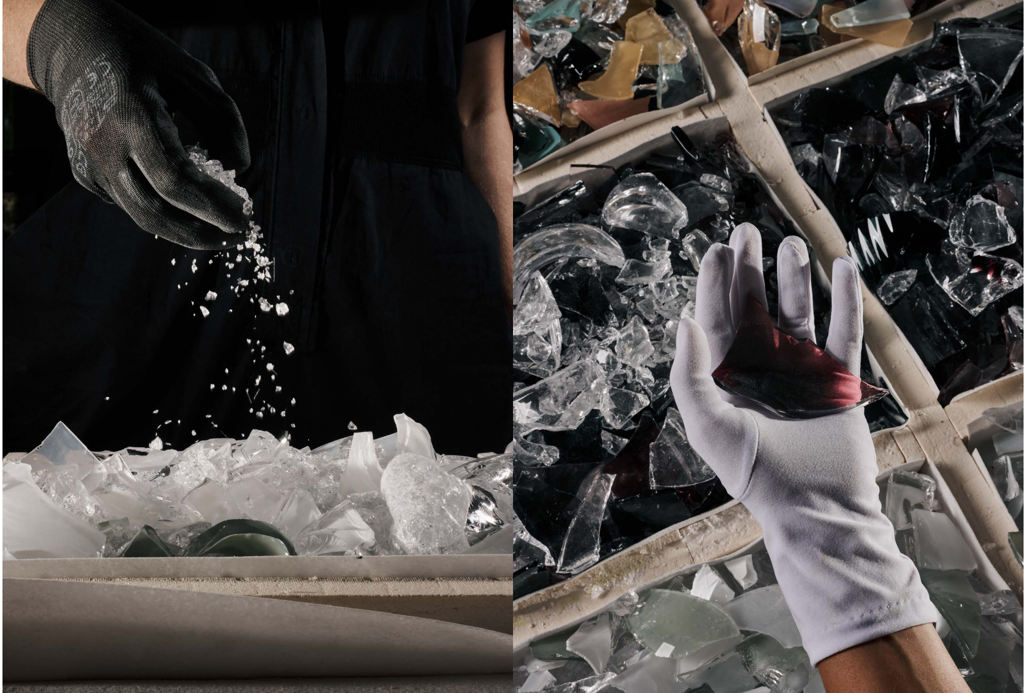
Each Fragmentglass panel is carefully assembled by stacking glass shards into a melting mold.
