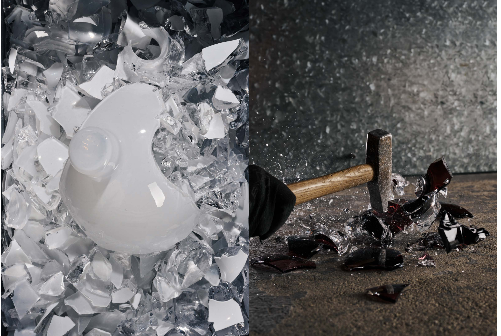
Fragmentglass is a new material that upcycles glass shards that failed to pass strict quality control of BOMMA's crystal lighting.
